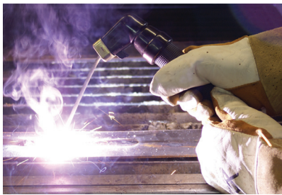
6) Hold the electrode slightly above the work piece to maintain the arc while travelling at an even speed to create an even weld deposition.
